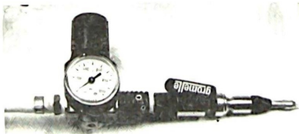
Fig. 1 The oxygen injector system used showing the pressure control value and the hand toggle switch.
